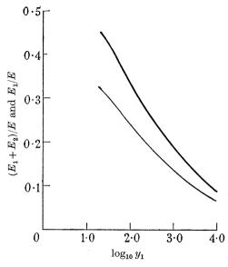
FIGURE 3. Heavy line,  $(E_1+E_2)/E$ ; thin line  $E_1/E$ .  $(E_1+E_2)/E$  is the proportion of the initial energy which is no longer available for doing work in propagation.  $E_2/E$  is the work done by heated air expanding against atmospheric pressure (see note added October 1949 (p. 172)).
