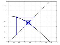
Iteration #7: p = 0.71278594551835,  $\cos(p) = 0.75654296195845$  p = 0.75654296195845Figure produces a **Cobweb**
