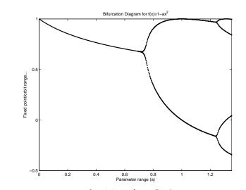
We see how iterations of  $f_a(x)$  go from fixed-points, to 2-orbits, to 4-orbits...
