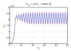
Simulation oscillates about the carrying capacity with period 2 behavior
