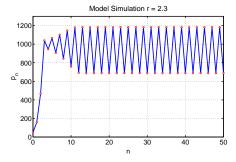
Simulation oscillates with period 2 about carrying capacity
